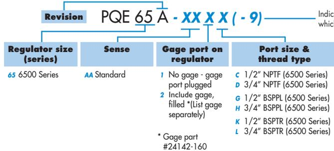
Indicates unit is to be assembled with PPC, which is ordered separately
